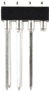
1. Cut the leg at the shoulder, of pin 4 of the 8-pin wire-wrap socket for U201 - see image at left
