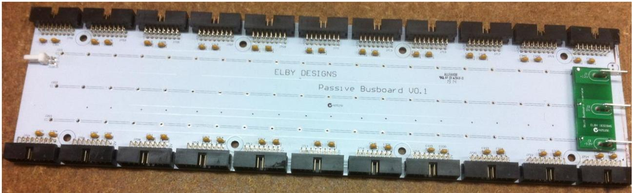
The ED703 is a low-height passive busboard similar to many other busboards on the market in that its sole function is to distribute the euro-synth power supply rails and control voltages throughout your system.
