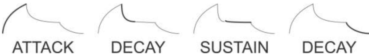
Figure 3 - Envelope stages. NOTE: The [DECAY] control defines BOTH falling slopes
