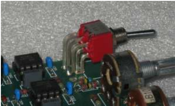
Nearest 2 legs of S101 have been removed by cutting them to about 5mm above the pcb
