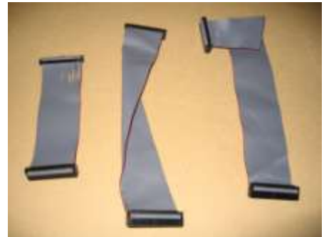
Main pcb – Panel pcb interconnect cables
