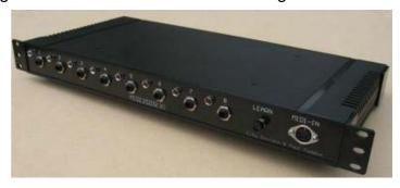
It also has a 'LEARN' mode, which lets you assign different notes and channels to different triggers. You could, for example, have four triggers on channel 10, two on channel 11, one on channel 15 and one on channel 2.
