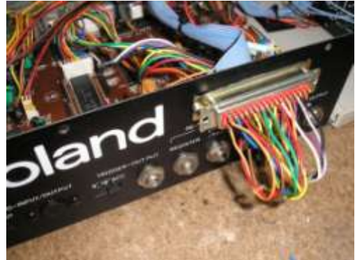
Example of an 'external connector'. Here it is shown with a loop-back plug fitted to restore normal operation of the equipment.
