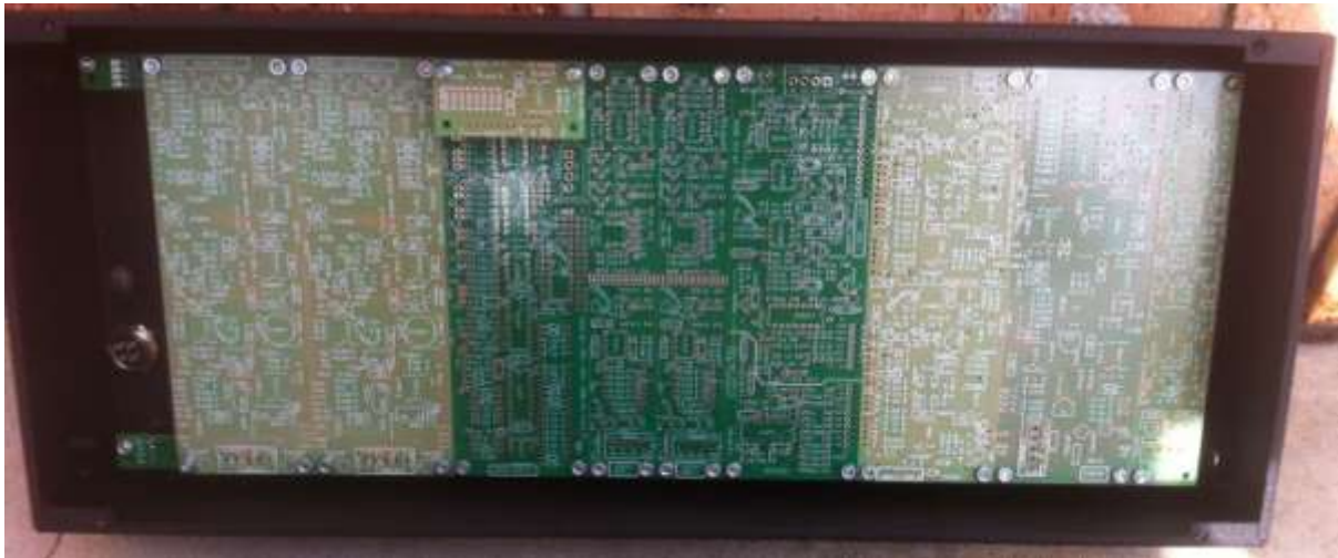
BOG PCB Set mounted on CGS91 PCBs
