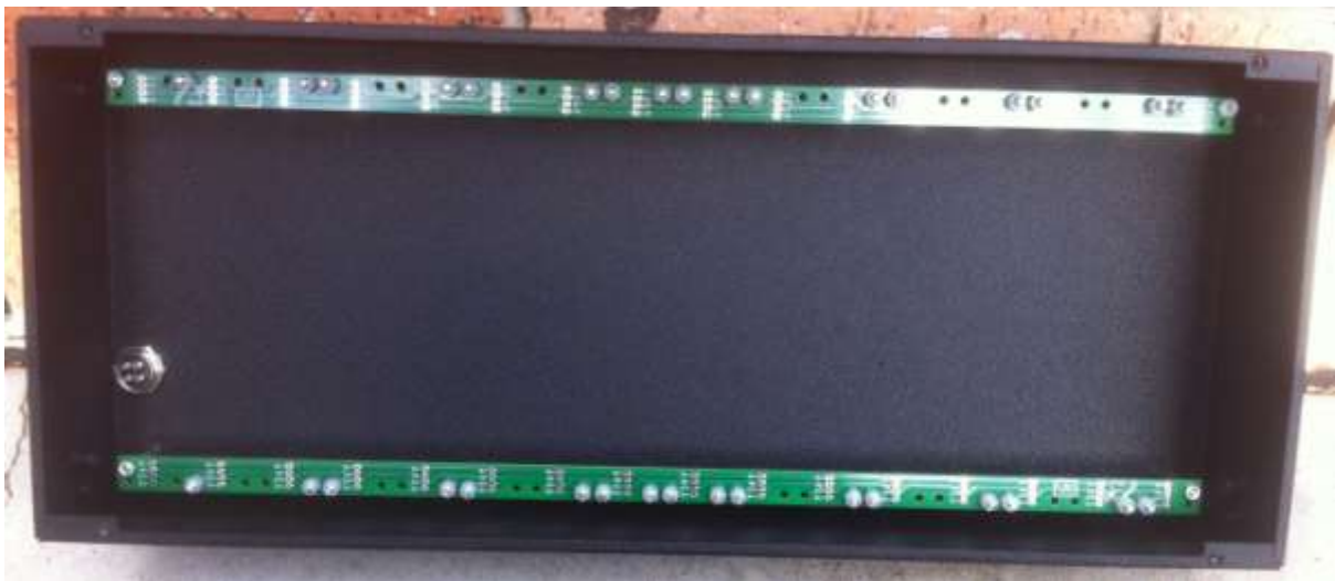
A pair of CGS91 boards mounted in our 4U Boat mounted and loaded with bolts and spacers for (in this instance) the BOG PCB Set.
