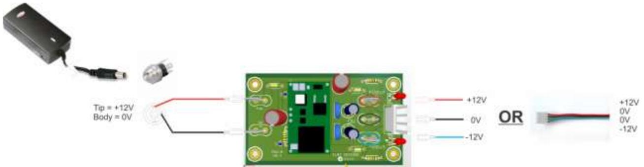
The above drawing shows the recommended connections for the PSU-8
