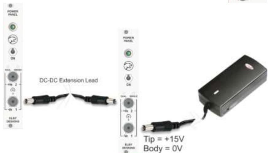
**NB: You must NOT connect multiple external power supplies to these DC sockets**
