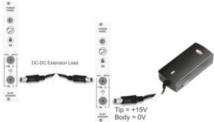
The maximum rating is approximately 5A (defined by the DC sockets) so this must be considered when connecting multiple power boards (this 5A figure is the total for both the +12V and -12V rails and should include a small allowance for peak loads).
