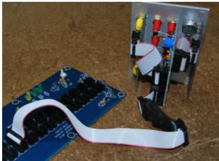
The EURO-5V Adaptor installed
