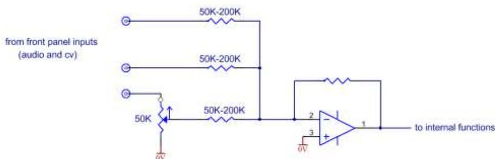
Figure 8.2 - Typical input network on Euro-Serge modules
