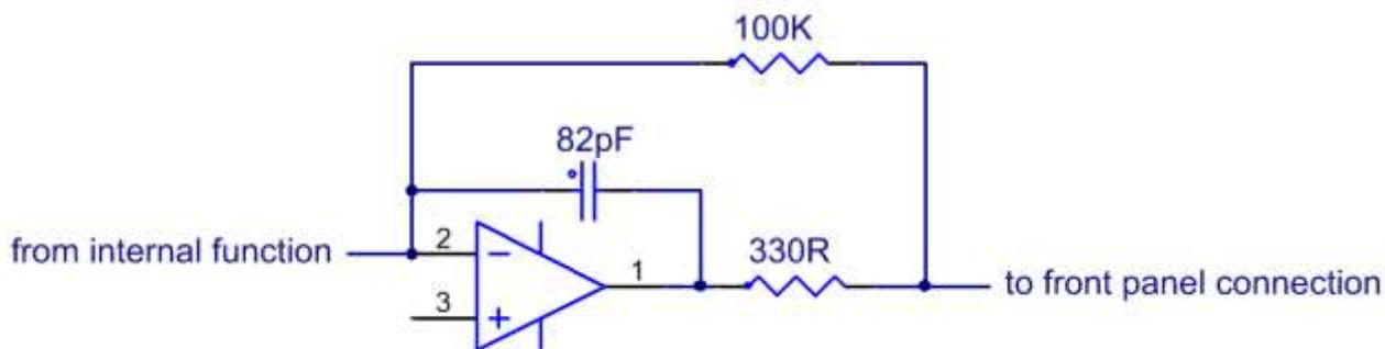
*Figure 8.1 - Typical output buffer in Euro-Serge modules*
