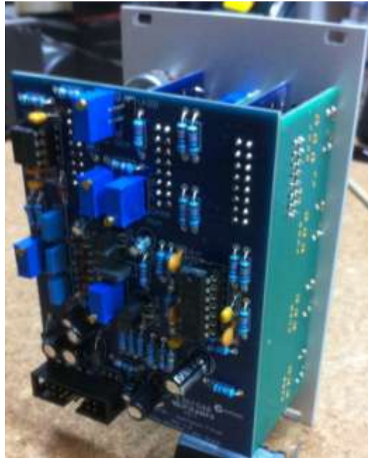
Figure 1.25 - Behind a typical Euro-Serge module.
