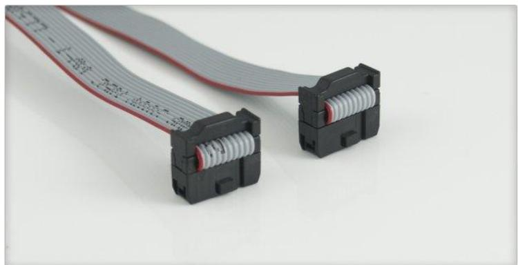
*Figure 1 - Correctly terminated IDC cable*
